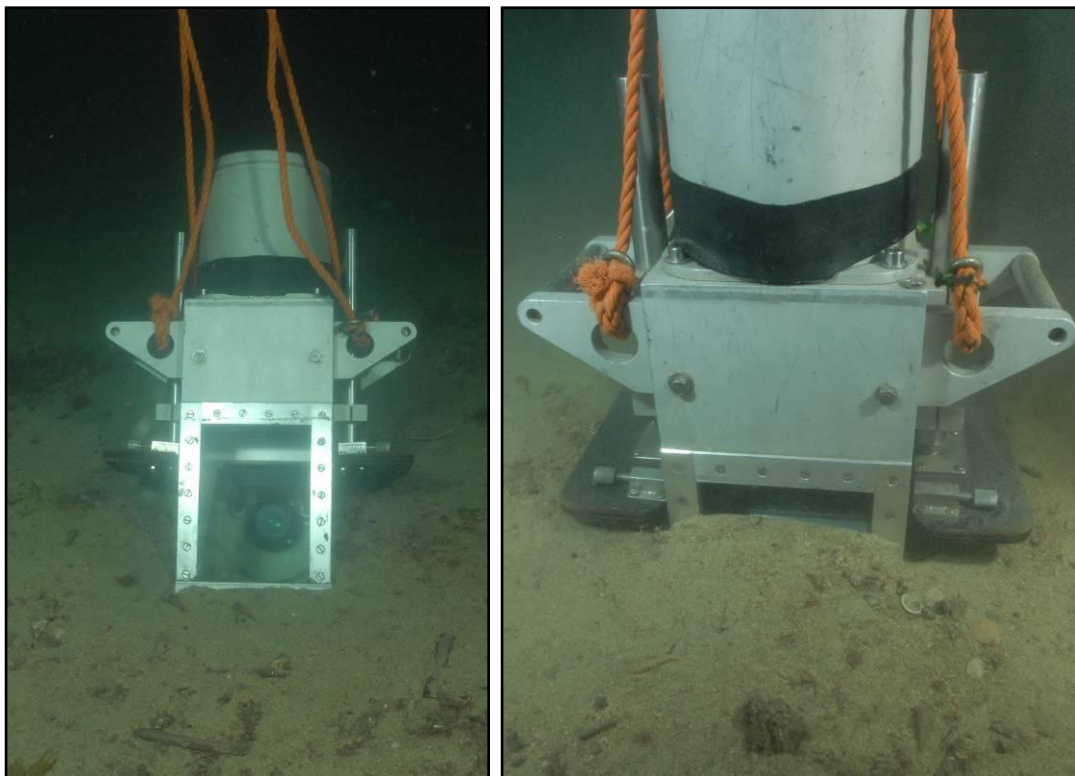
Figure 2.2: Diver operated Sediment Profile Imaging camera. The left-hand image gives a view of the camera at the sediment surface. The right-and image shows the SPI camera when inserted into the sediment
